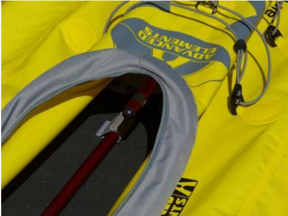
Locate the sleeve on the “underside” of the top bow hull. Take pole #4 and push it through the sleeve, and guide it into the top bow tube. Make sure the rounded side is facing the cockpit. Frame is now done!
