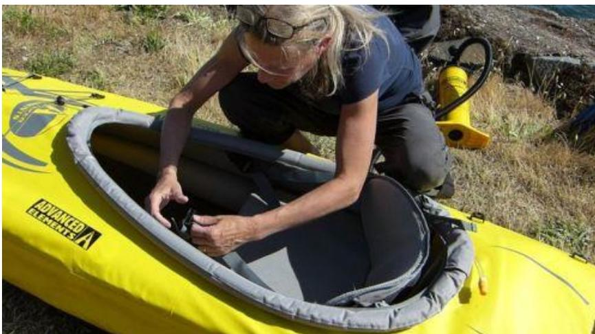
Position the seat at the “edge” of the floor cushion and attach the seat utilizing two forward clips and two rear clips. Do not put the seat farther back, as it will upset the balance – if you need more legroom, partially deflate and adjust the front thwart.
