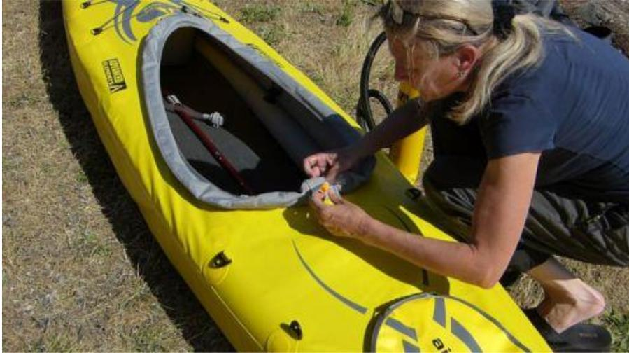
Inflate the coaming tube to 1 PSI using the Boston valve adaptor OVER the twist lok. This helps keep water from running into the seating well.
