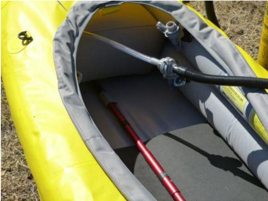
Next position and pump up the thwarts. This is probably the most critical step in the process to ensure a balanced setup. Line up the rear thwart with the line printed on the kayak body. It is important to keep the rear thwart at full inflation of 2 PSI; its function is to spread the sides, and the full airbag is used in weight capacity calculations. Make sure the thwarts/airbags are even across the floor, and the side chambers even with the thwarts.
