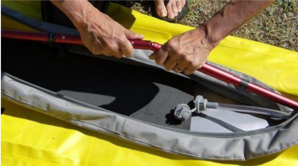
Push down on both pole #1 and #2 until they pop into position, forming one long pole.
