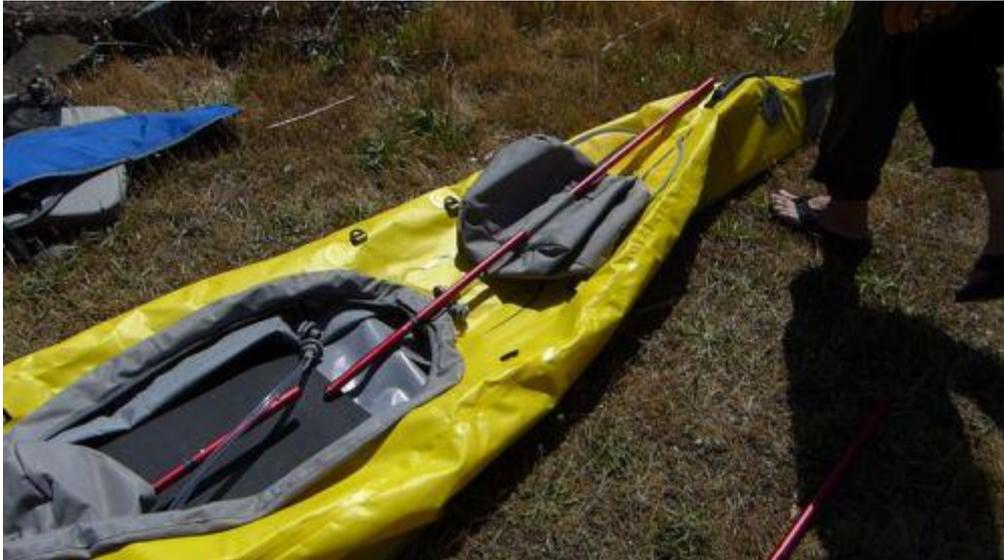
Next insert pole #2. Once again, push this through the sleeve on the bottom of the rear thwart, with the number facing the cockpit. Then insert the thwart into the stern of the kayak, also with pole side down. Open up the rear hatch cover, and push the velcro out of the way to locate the rear bottom tube. Again, insert pole 2 into the stationary bottom tube opening.
