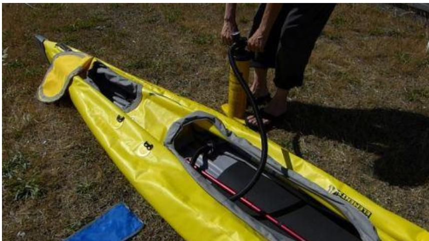
Partially inflate the four side chambers, starting with the lower bladders – about 7 pumps each will give it some shape.
