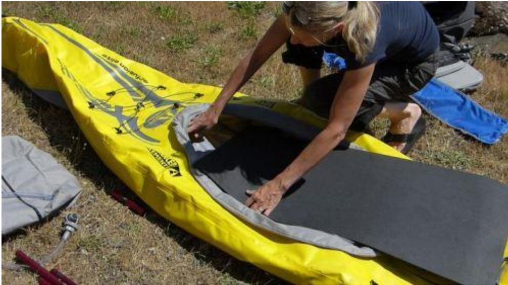
Next, put the foam floor into position by setting the wider end in the cockpit – this will position the small rectangular cutout over the velcro tabs in the floor. Make sure you pull the velcro tab through the cutout. Tip: the foam floor only covers the area where your feet rest.
